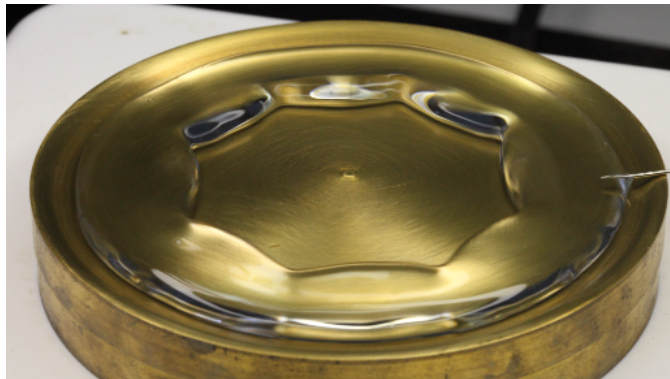
Figure : Photograph of the water torus levitated by Leidenfrost effect. The internal surface of the ring destabilizes spontaneously to form a rotating polygonal shape
